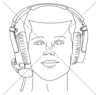
Figure 3: Incorrect Mic Position
